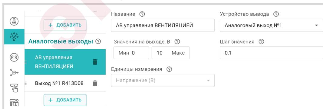
The screenshot shows a configuration window for an analog output. On the left, there is a sidebar with a list of outputs under the heading "Аналоговые выходы". One output is selected: "АВ управления ВЕНТИЛЯЦИЕЙ". Below it, another output "Выход №1 R413D08" is visible. A "+ ДОБАВИТЬ" button is at the bottom of the sidebar. The main area contains the following fields:
