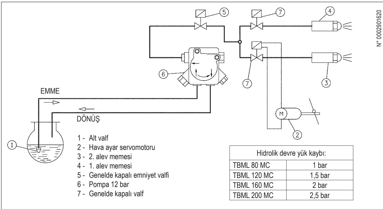
**TBML 80 MC BORULARI BOYUT ŞEMASI**
